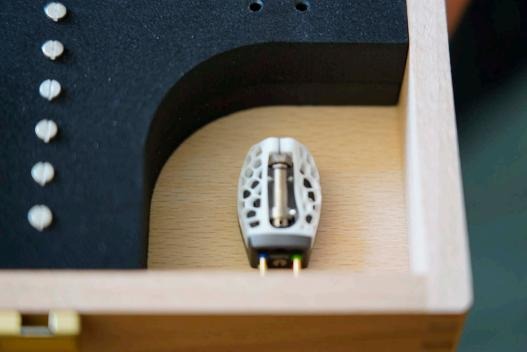
Requisite Finest MC cartridge with patented monobloc-ceramic transducer
